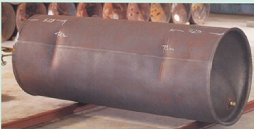
No leakage during prototype testing of ISGEC Container dropped on 2 Iron rails from a height of 20 feet.
